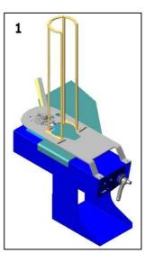
underneath the top of the stands by fastening it with two M6 bolts (if applicable). The opening in the plate has to be towards the rear side (**picture**).
